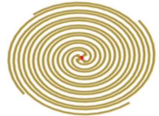
Self-complementary 4-arm Archimedean spiral antenna
