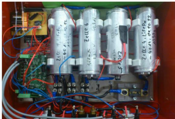
Four LiFePO<sub>4</sub> cells with BMS and safety circuits as a car starter battery
